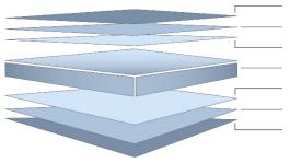
Finish Coat (Finish Coat + Primer = nominal 25µm) {Refer Notes 1, 4 & 5} Universal Corrosion Inhibitive Primer Conversion Coating Aluminium / Zinc / Magnesium alloy-coated steel with Activate® technology substrate (fence panels) or zinc-coated steel substrate (post & rails) Conversion Coating Universal Corrosion Inhibitive Primer Backing Coat (Backing Coat + Primer = nominal 25µm total for panels or nominal 10µm for post & rails) {Refer Note 6}
